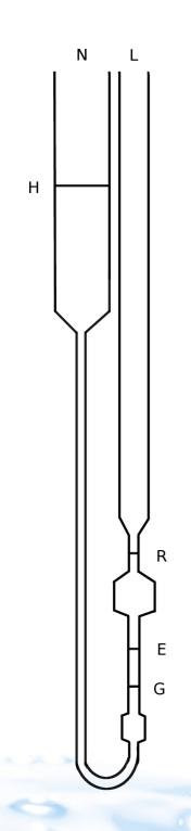
Use a rubber bung fitted with a glass tube and stopcock to apply slight, controllable, excess pressure to tube L.
